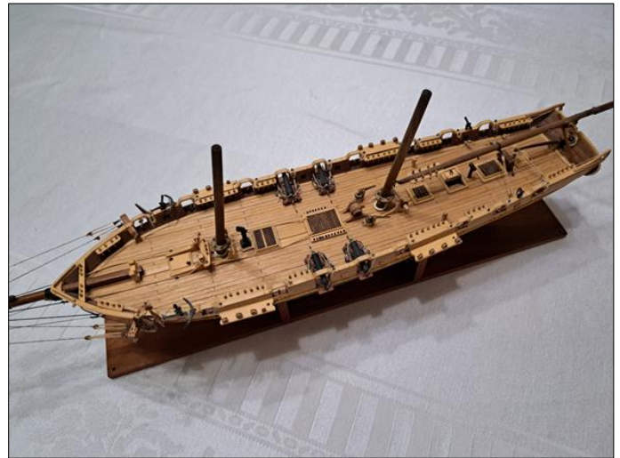
"Grecian" Baltimore Clipper. Carved solid hull veneered with Boxwood, Tanganika, Mahogany, Gabon Ebony. Finished as described with amber and blonde shellac.
